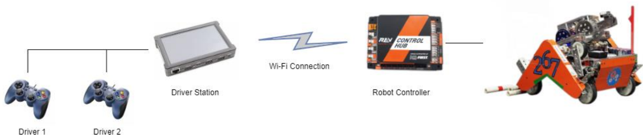
Figure 2: Point-to-point connection between the robot controller and driver station.
