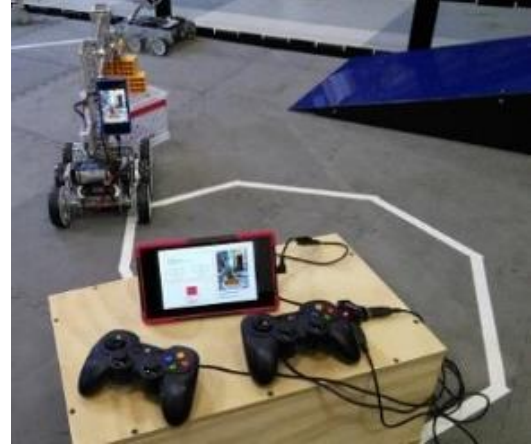
Figure 1: Driver Station Device connected wirelessly to a FIRST Tech Challenge Robot
