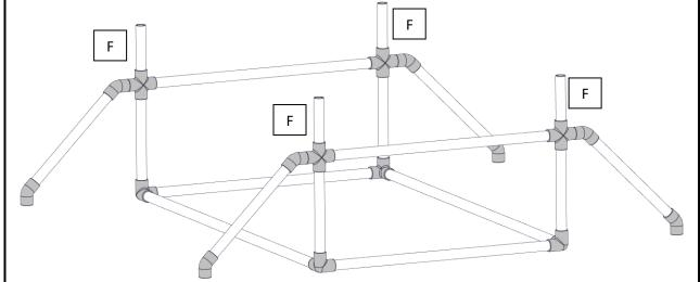
Tap [4] tee fittings onto [2] part As. Place the assemblies on top of the part Fs placed in Step 7. Ensure the top of each Part A is 20" from the floor.
