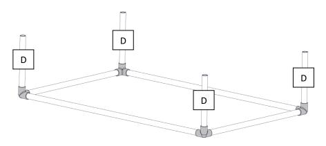
Create [2] assemblies, each with [1] part B and [1] cross fitting at either end. Attach them to the larger assembly at the locations where the part Ds were placed in Step 3, as shown. Ensure the top of each Part B is 13" from the floor.
