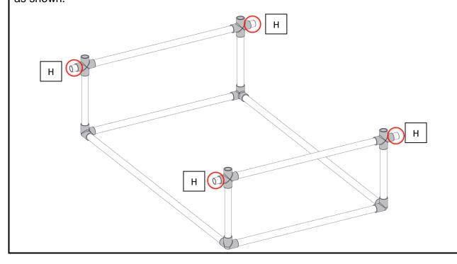
Create [4] outrigger assemblies, each with [1] part C and [1] 45 degree fitting at either end. Ensure the fittings are rotated such that they occupy the same plane, as shown. Attach them to the larger assembly at the locations where part Hs were placed in Step 5. These should touch the ground.
