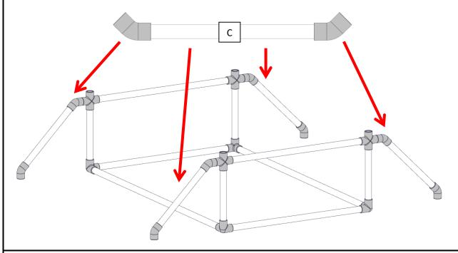
Step 7 Insert [4] part Fs into the open slots on the cross fittings, as shown.
